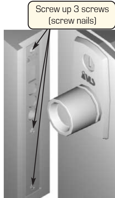
Figure 17 – Installation of the strike plate
